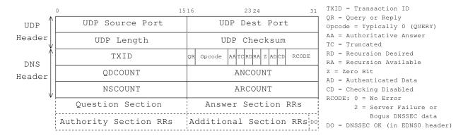
Figure 2. DNS and DNSSEC packet format. DO bit is in EDNS0 Header in Additional Section RR
