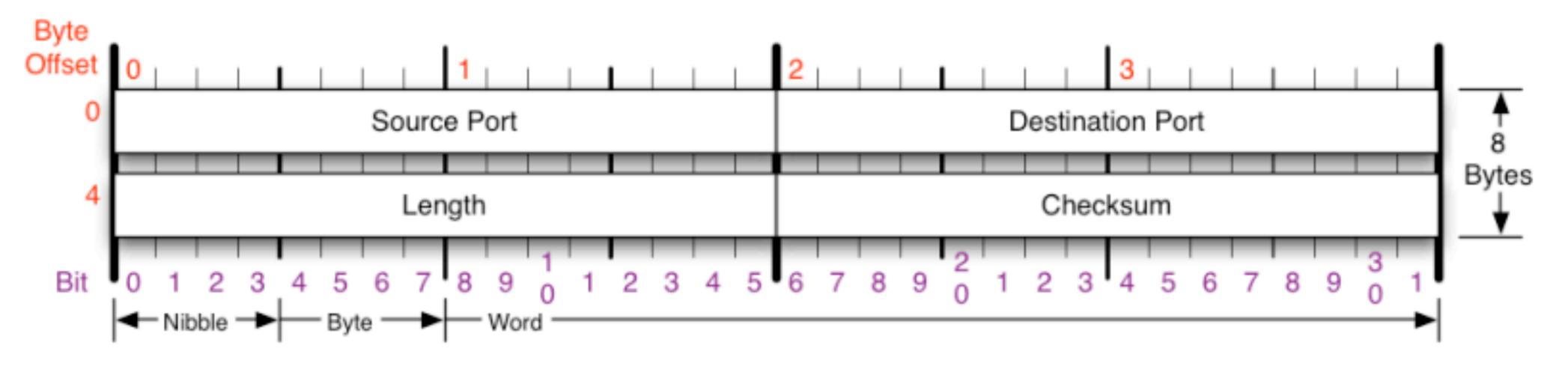
Example: What bytes contain each field in a packet header
